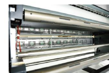
Inflatable take up and feed media shaft.
