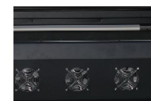
Integrated IR & cooling fan system.
